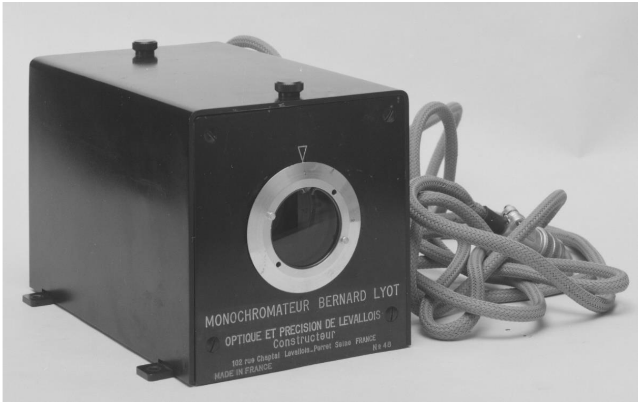
Figure 14 : The Lyot filter ( 0.75 \text{ \AA} FWHM) manufactured by the OPL company. Courtesy Paris observatory.
